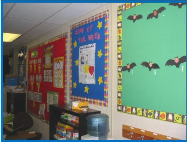
This is an acceptable display meeting the requirements of 3(a). Paper is .025 inches thick or less and is secured flat up against the wall. It does not protrude or curl away from the wall.
