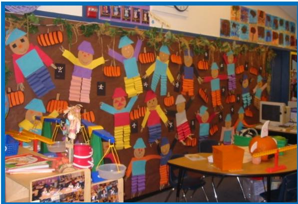
This would not be an acceptable display under 3(a) as the decorations protrude away from the wall. Even if the material was treated with a fire retardant, this display would exceed the maximum 10% limit of the display area as per 3(c).
